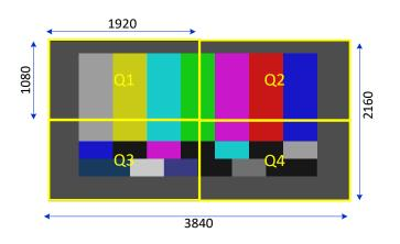
Each quadrant is delivered over an independent **3G-SDI**, **SMPTE ST 425-5** link to the HEVC encoder. Each quadrant will be encoded by using standard parameters described in this document; the Dolby-E will be injected in Q1.
